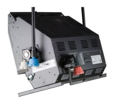
Arturo 2 is a 2500W dual power softlights with two lamps, switched individually, to give intensity control with constant colour temperature. It provides virtually shadowless diffused illumination. The asymmetric beam distribution offers a constant and even illumination.
