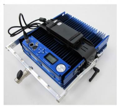
This bracket fits onto the back of the Creamsource Mini fixture and allows the power supply to be securily attached, simplifying rigging in studio applications. Velcro straps are supplied to attach the power supply onto the frame. Constructed from bent aluminium with black powder coating.
